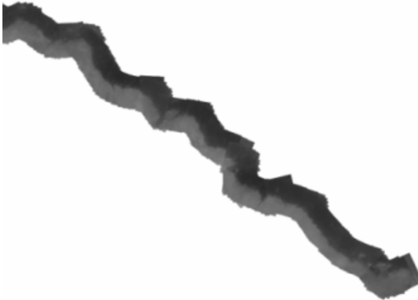
Figure 3: A mosaic showing the ROV in contour tracking mode along the outer boundary of a bank of dead maerl.
