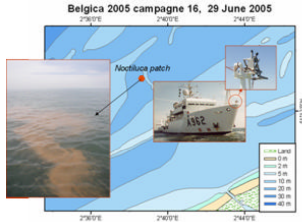
Figure 3: Position of the Noctiluca patch encountered by RV Belgica on 29 June 2005 and measured by a combination of 3 TriOS-RAMSES radiance sensors and ac9 absorption and scattering meter.
